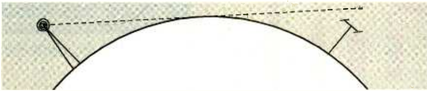
FIG. 5 —REGARDLESS OF MANUFACTURER OR DEALER claims to the contrary, unless both the transmitting and receiving antennas are located quite high, reliable terrestrial reception is limited to 60 miles or less because of the curvature of the Earth.
