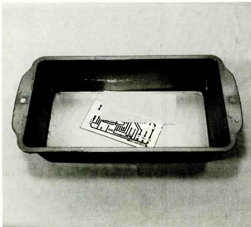
After ironing, paper-based TTPs are soaked in water to remove the paper from the PCB. Be patient as peeling the paper before it has soaked off could produce poor results.
