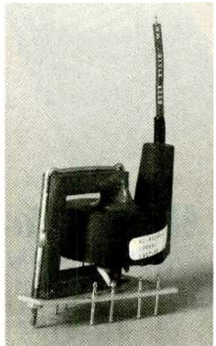
Here is a standard television-flyback transformer. Modifying it by adding a new primary winding is the heart of the Poor Man's Plasma Globe.
